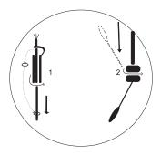
Peel the plastic ring off the counterweight before installation and set the ring around the cable then insert the cable from the conic part into the counterweight and fix it with moderate pressure at the fixing end.
