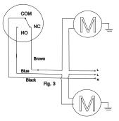
This shows the auto-switch between filling and emptying water , which is an extension of the two basic functions.
